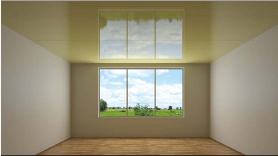
Seams are parallel to the window opening. The PVC film should start from the window. The first seam should be on maximal distance from the window.
