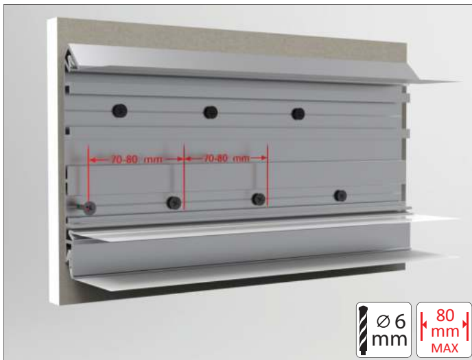
Fastening the profile to the plasterboard wall
