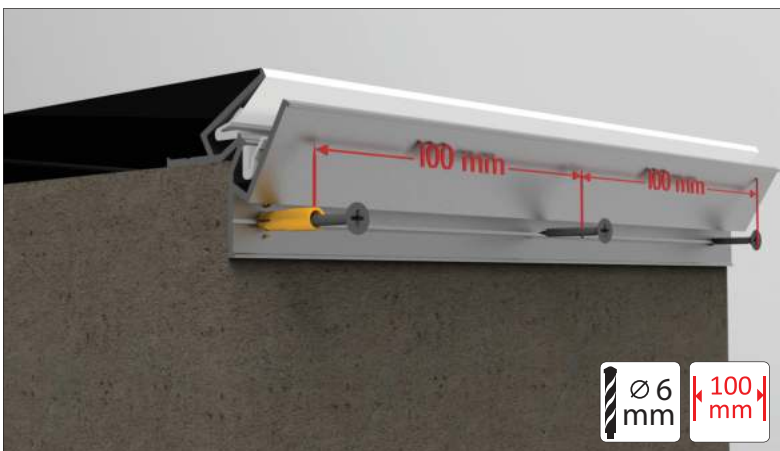
Fastening the profile to the concrete
