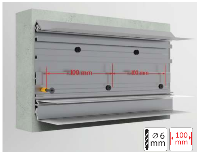
Fastening the profile to the concrete wall
