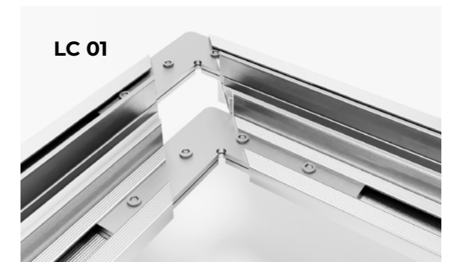
LC 01 for corners: 4 plates (2 plates / 1 slot) + 8 bolts
