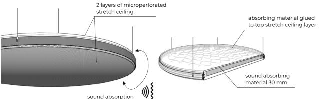
To create acoustic panels, a mould of AL19 profile, 2 layers of stretch ceiling and 30 mm thick sound absorbing material are used.
