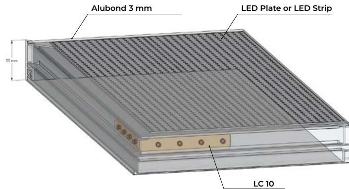
This profile is a special solution for cases where light panels with minimal thickness but effective luminous flux are required. Despite its light weight, this profile is strong enough to create frames of various sizes. The minimum size on one side of the frame can be 20 cm, which makes it possible to create light, narrow, but at the same time long luminaires.
